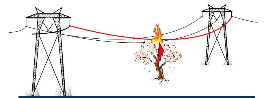
High temperatures can damage line material or cause line to sag too low, creating safety hazards and/or outages.
